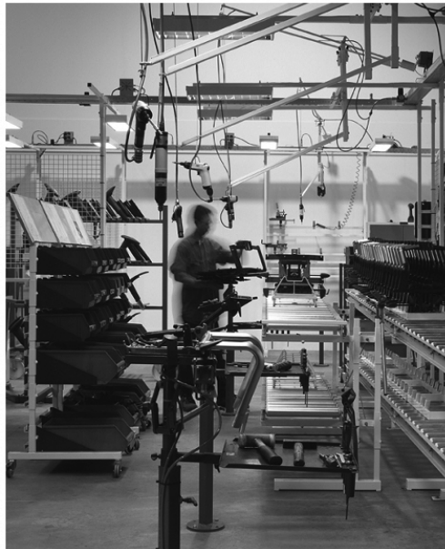
Figure 1: Recycling station at BMA Ergonomics. Chairs are disassembled at end of life cycle using the same (common) hand tools and workstation aids that were used to assemble the product
