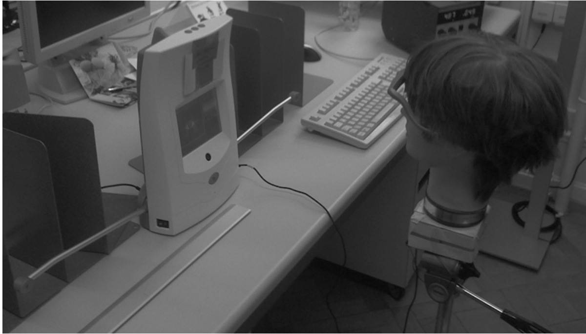
Figure 1: The testing system (VisioPrint) used in Menozzi et al. (2008) to record an individual's preference for head and eye movements. Participants had to look at blinking LEDs (central, peripheral left, peripheral right) while wearing a frame that emitted an ultrasound
